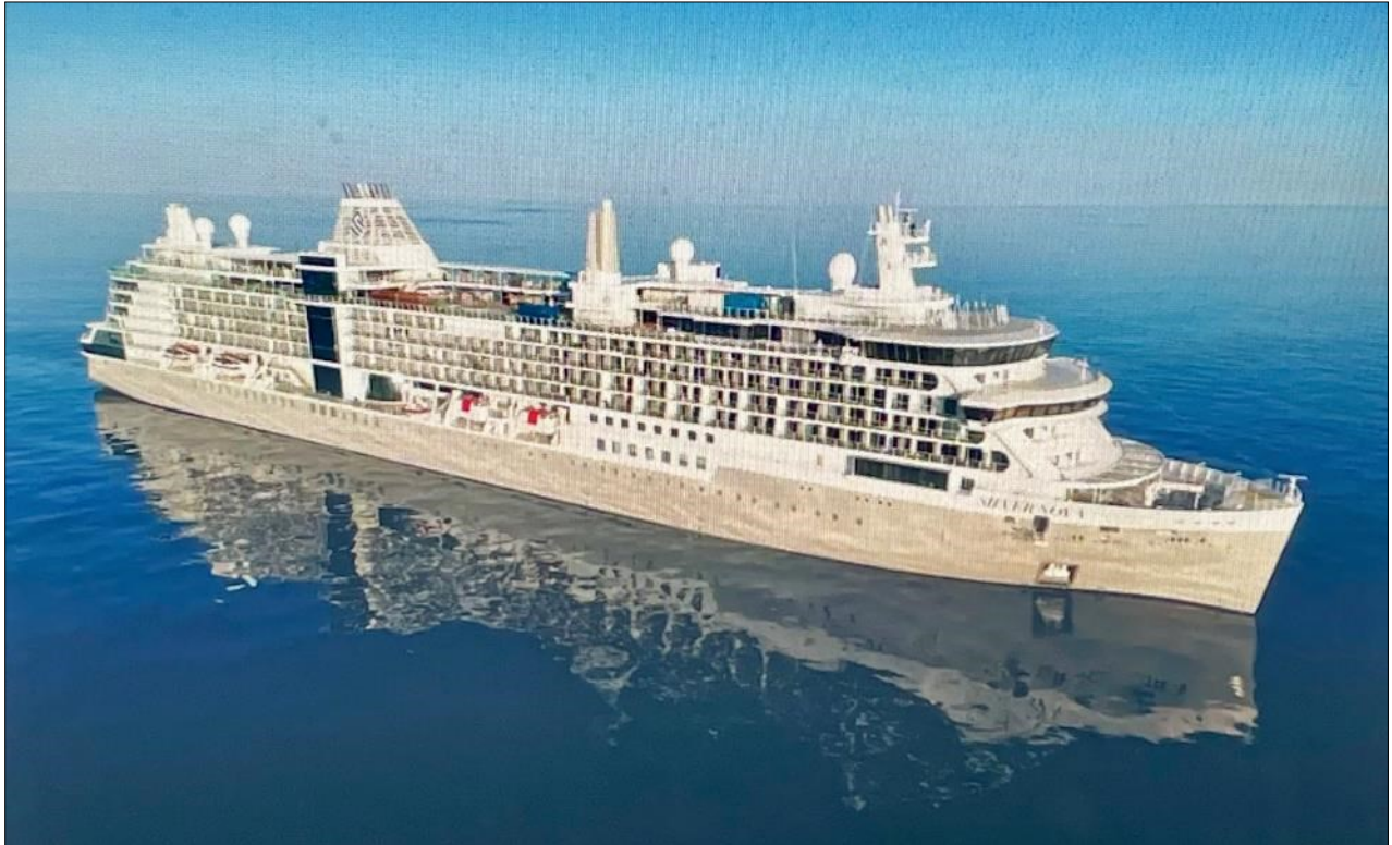
SILVER NOVA's funnel and amidships ventilation tower are not on the ship's centerline but are offset for structural and layout reasons. A glass enclosed elevator is visible adjacent to the funnel. (Silversea Cruises)
