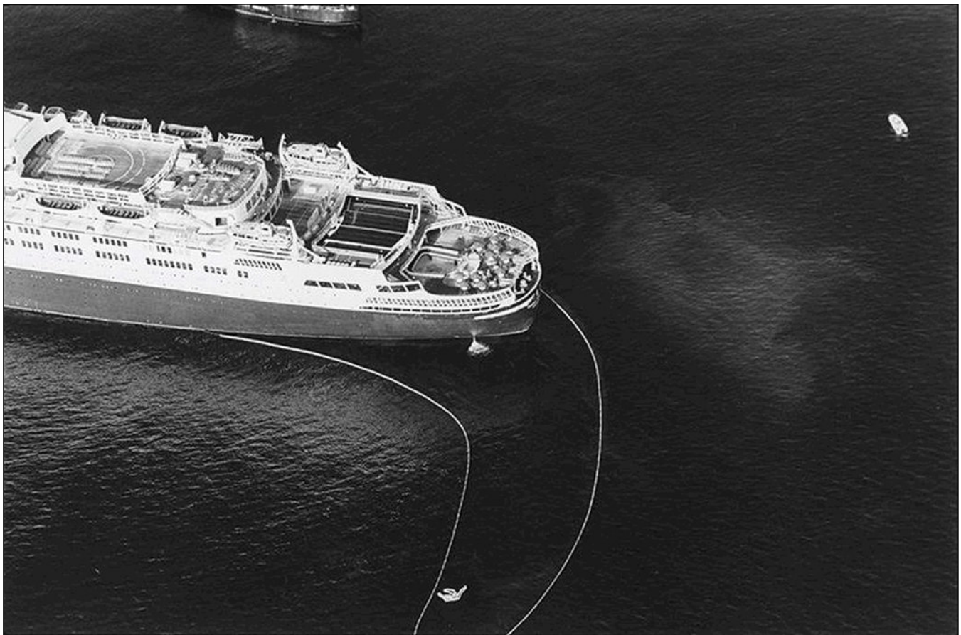
Booms were swung from the stern to contain oil spills, such as the patch seen outside the containment area, at right.
