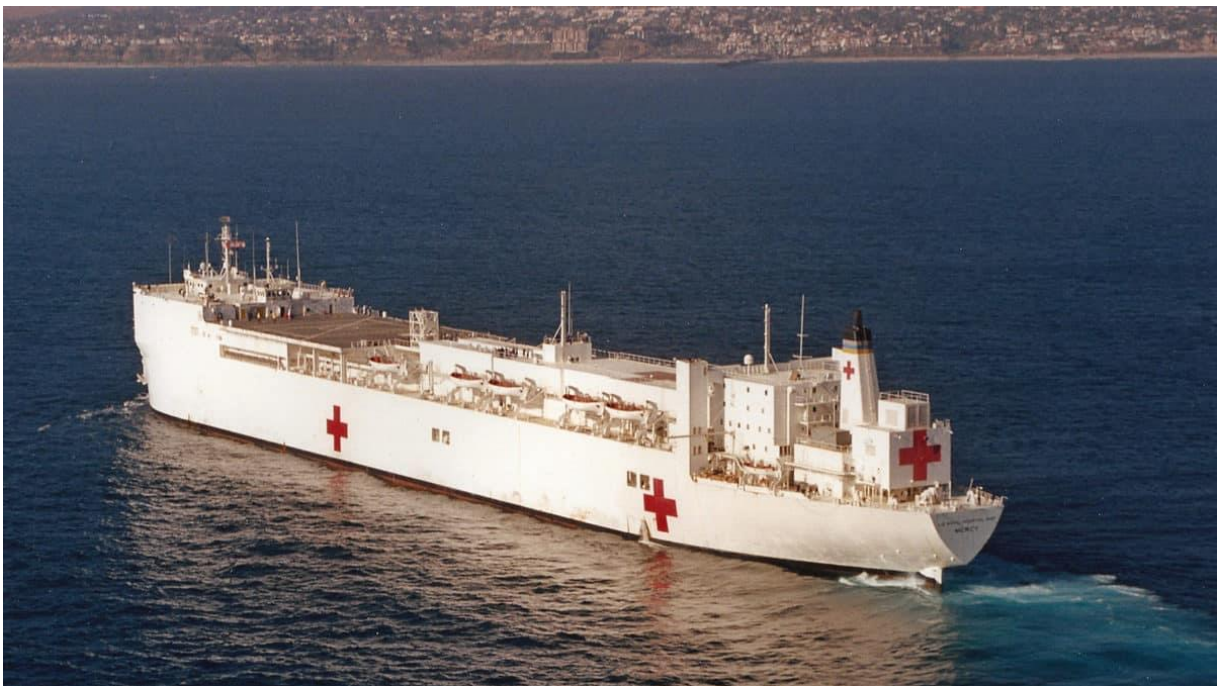
USNS Mercy, formerly the steam tanker Worth. Note the helicopter pad and the tanker's deck house at stern, which was incorporated into the deck structure. (Photo Courtesy: Capt. James McNamara)
