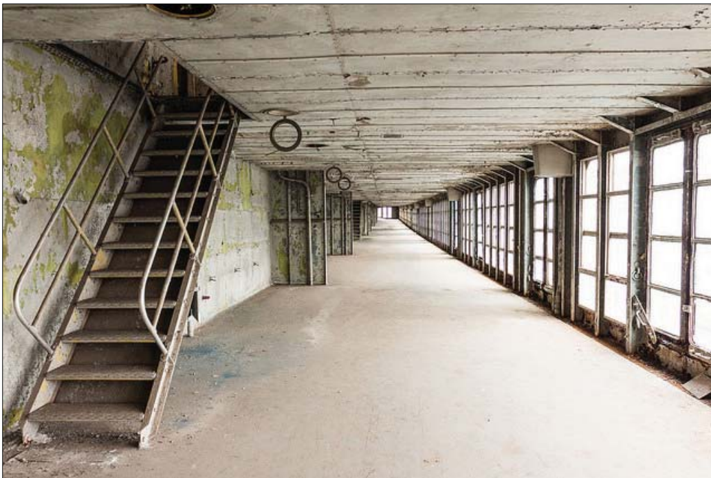
The First Class Promenade Deck had plenty of room for deckchairs and strollers, all of whom could gaze over the Atlantic Ocean through full-height windows. The glazing was fitted with escape doors, for boarding lifeboats in case of an emergency. (Doug Newman)
