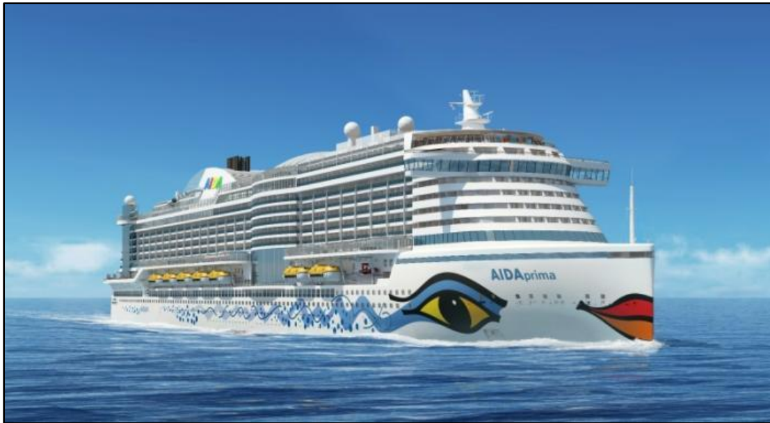
The knife-like stem of AIDAPRIMA is reminiscent of early 20th century liners, while her massive superstructure is clearly 21 st century design.
