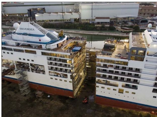
SILVER SPIRIT was cut in half for expansion at Fincantieri Shipyard, Palermo, Italy (Silversea/Fincantieri)
