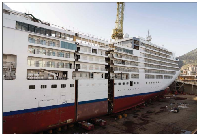
SILVER SPIRIT was cut in half for expansion at Fincantieri Shipyard, Palermo, Italy (Silversea/Fincantieri)
